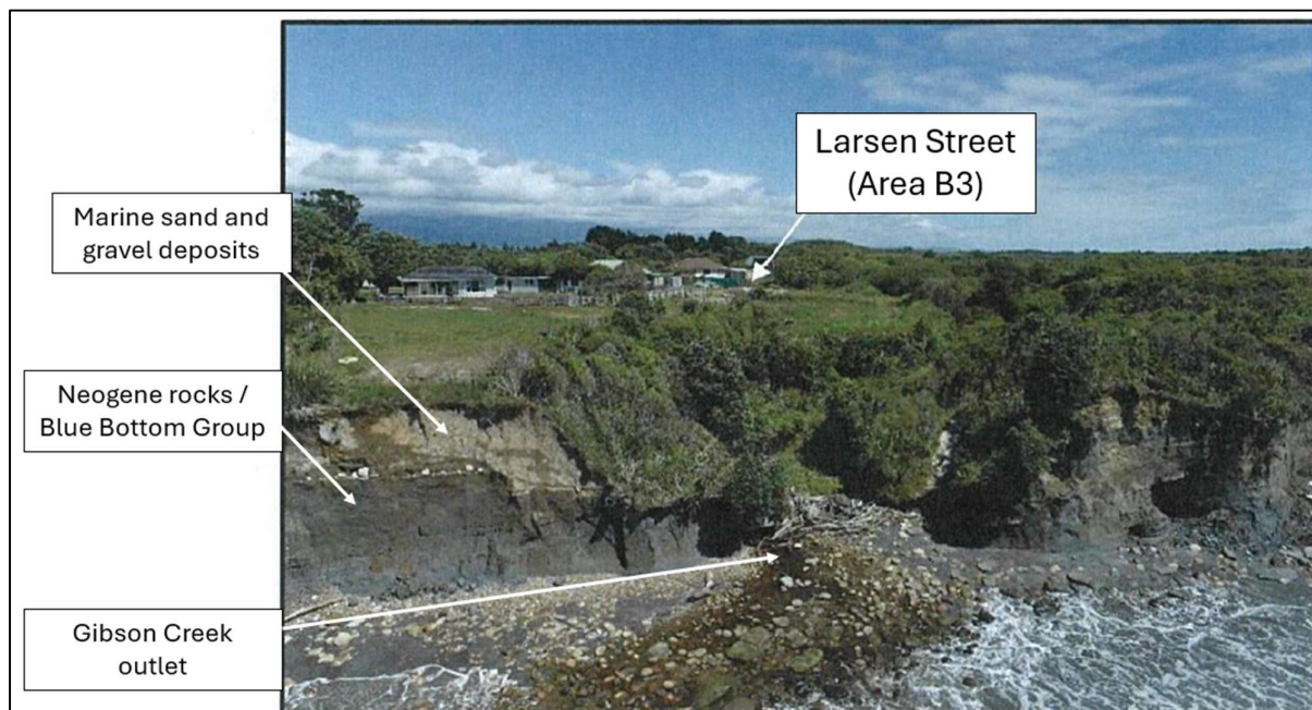
Figure 5.4: Oblique aerial view showing cliff edge overlooking the Tasman Sea (Buller Bay) and Gibson creek Outlet. Photo sourced from Davis Ogilvie (2023) and annotated by BTW
