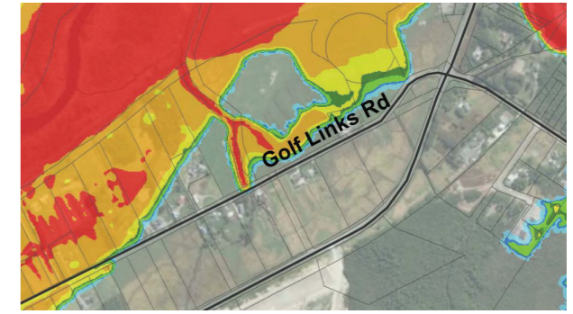
Figure 2. 1 in 100 year event including climate change (2100) RCP Scenario 8.5, 1.4m Sea Level Rise, 0.4m Storm Surge
