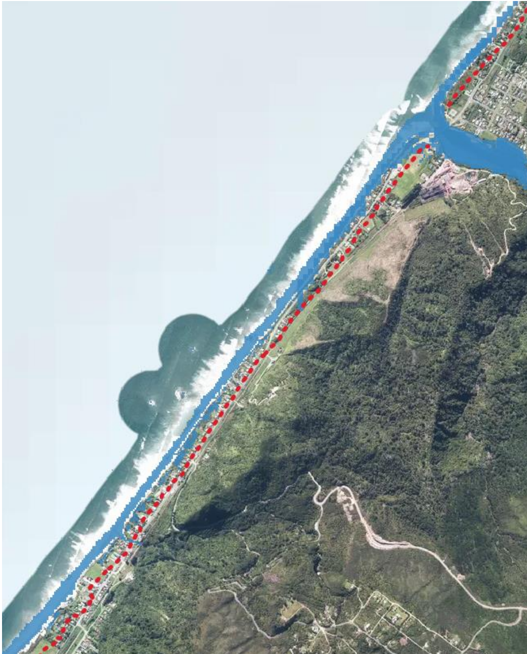
Figure 4-8: 1% AEP storm-tide+wave setup for present sea level in Granity Hector and Ngakawau . Blue shading shows areas at risk of inundation. The dash red line show the area of coastal erosion hazard for a 100-year outlook.
