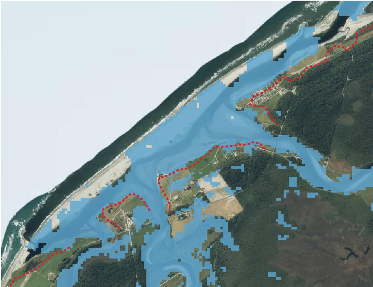
Figure 4-35: Okuru inundation extent from the 1%AEP storm-tide+ wave setup at present sea level. Blue shading shows the inundation extent and the red line shows the 100-year outlook coastal erosion hazard area limit.
