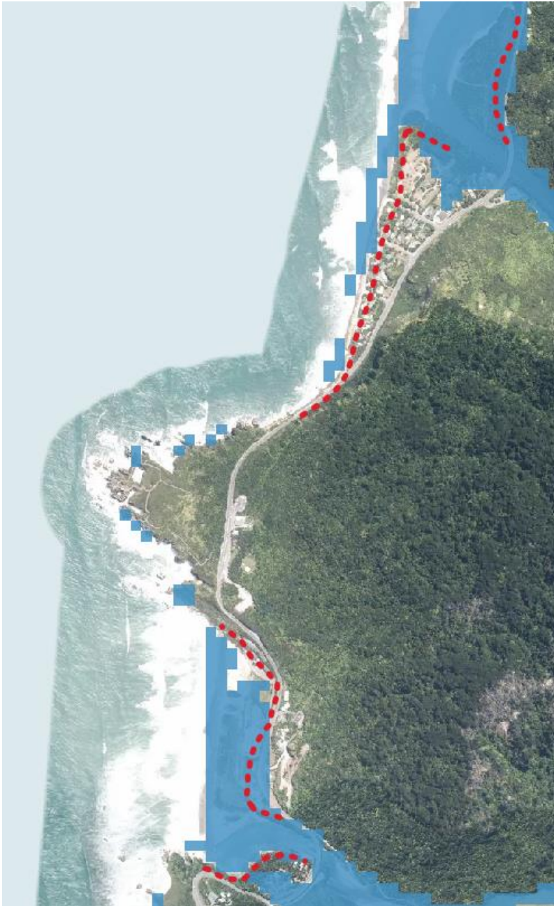
Figure 4-18: inundation extent from the 1%AEP storm-tide+ wave setup at present sea level for CHA 12 Punakaiki Village and CHA 13 Punakaiki River Beach. Blue shading shows the inundation extent and the red line shows the 100-year outlook coastal erosion hazard area limit.
