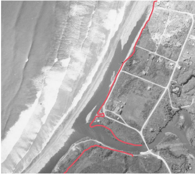
Figure 3-2: Georeferenced aerial image of Rapahoe in 1939 and the 2020 vegetation line (red line). Note the gravel barrier has rolled over and the narrow lagoon does not exist anymore. The gravel beach lies near the vegetation line and is depleted.
