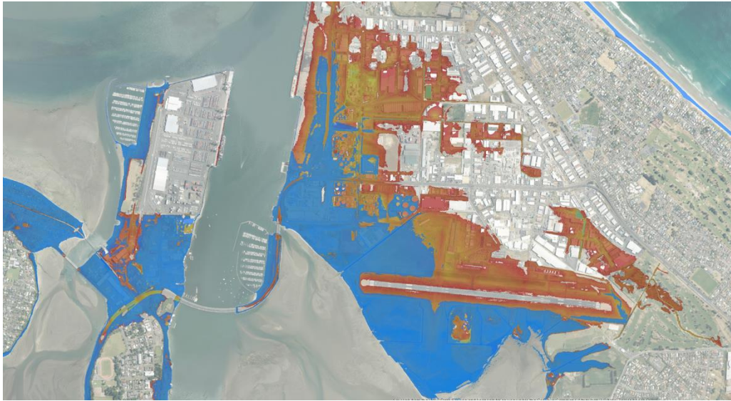
Figure 2-11: Example comparison of dynamic model of flooding (blue) with bathtub model (red) for Tauranga. The scenario modelled was a 1% AEP storm-tide + 1.25 m SLR. In this case the duration of high sea-levels is insufficient to spread floodwater to the full extent predicted by the bathtub model. Source: Reeve et al. 2019.
