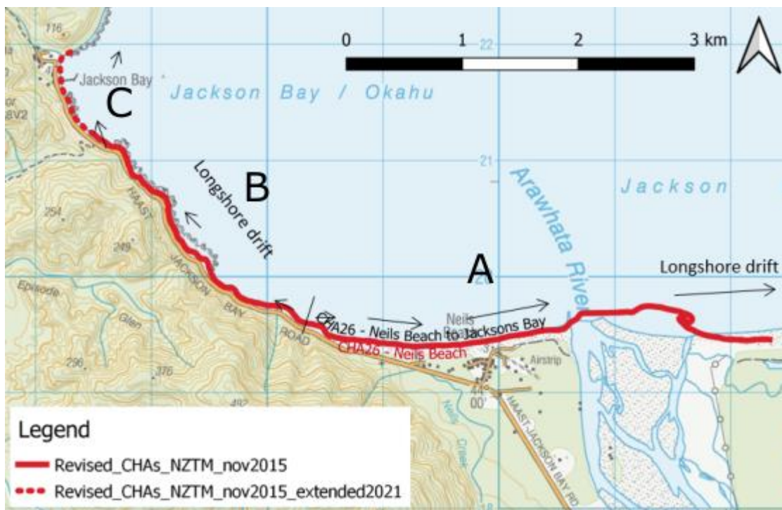
Figure 4-36: CHA26 Neils Beach to Jackson Bay. Arrows schematically indicate prevailing longshore drift direction and magnitude in the lee of Jackson Head. A, B and C correspond to three subsection of CHA26 [Map source: LINZ].
