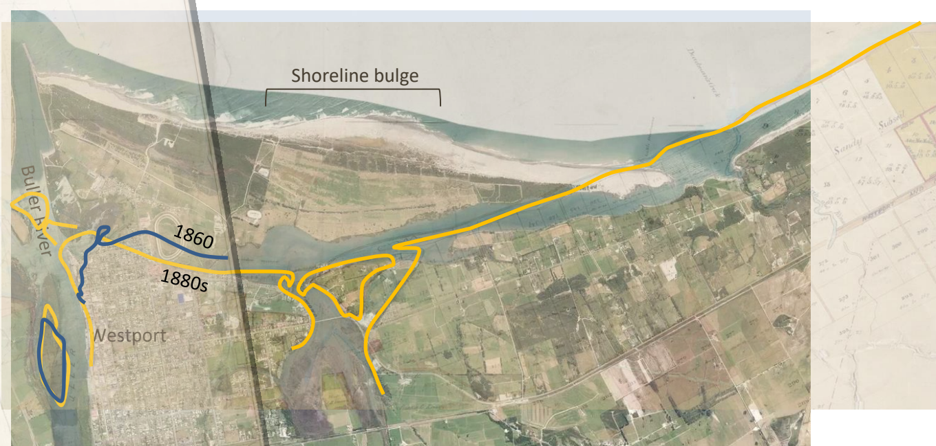
Figure 4-10: CHA4 Orowaiti Lagoon aerial photograph with 1860 shoreline. Orange/blue lines indicate shorelines and high-water mark from 1860s/1880s survey maps [Credits: Aerial photo – LINZ, shoreline digitised from NZ archives (ref: CH1031/SO 159 (1873), and Archway Record Code: R17224538 (1860)].
