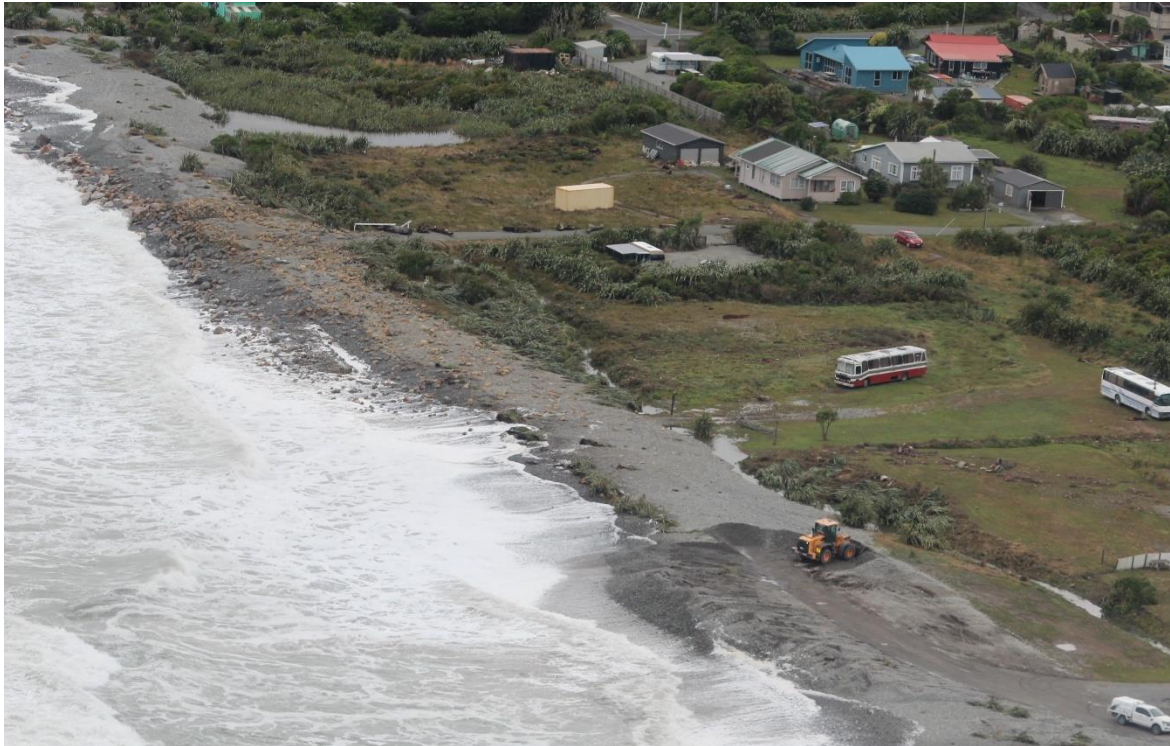
Figure 4-24: Aftermath of wave overwashing at Rapahoe following exTC Fehi. Note driftwood debris spread up to 50 m inland from the beach face, washover of gravel enveloping Beach road and spreading into flax bushes and flooding inundation of low-lying areas and blocking of drains. Also note the scattered rock from the damaged revetment. Note section with busses since infilled to increase land elevation. [Credit: WCRC].
