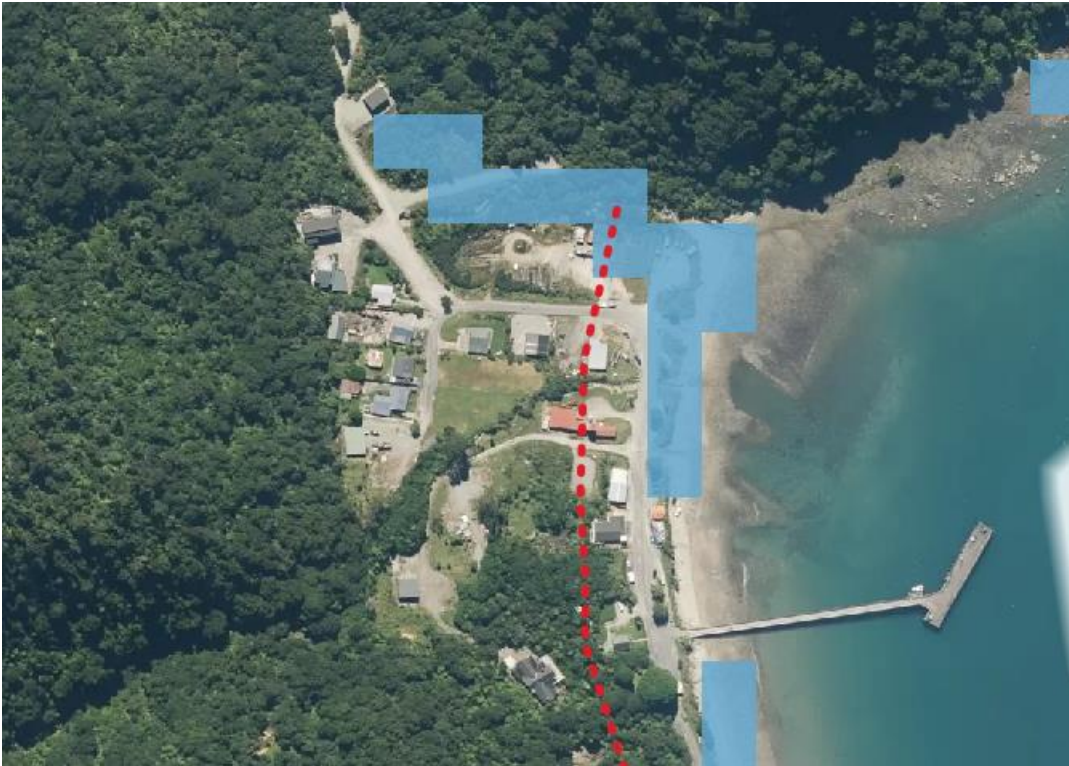
Figure 4-43: Jackson Bay inundation extent from the 1%AEP storm-tide+ wave setup at present sea level. Blue shading shows the inundation extent and the red line shows the 100-year outlook coastal erosion hazard area limit.
