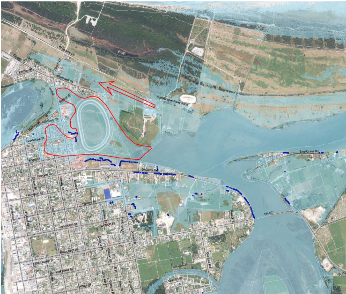
Figure 2-17: Validation of coastal inundation model for exTC Fehi. Blue dots show the location of surveyed flood debris marks, the red polygon area represents the inundation extent and flow direction observed by witnesses, blue shading represents simulated flooding from the hydrodynamic model.
