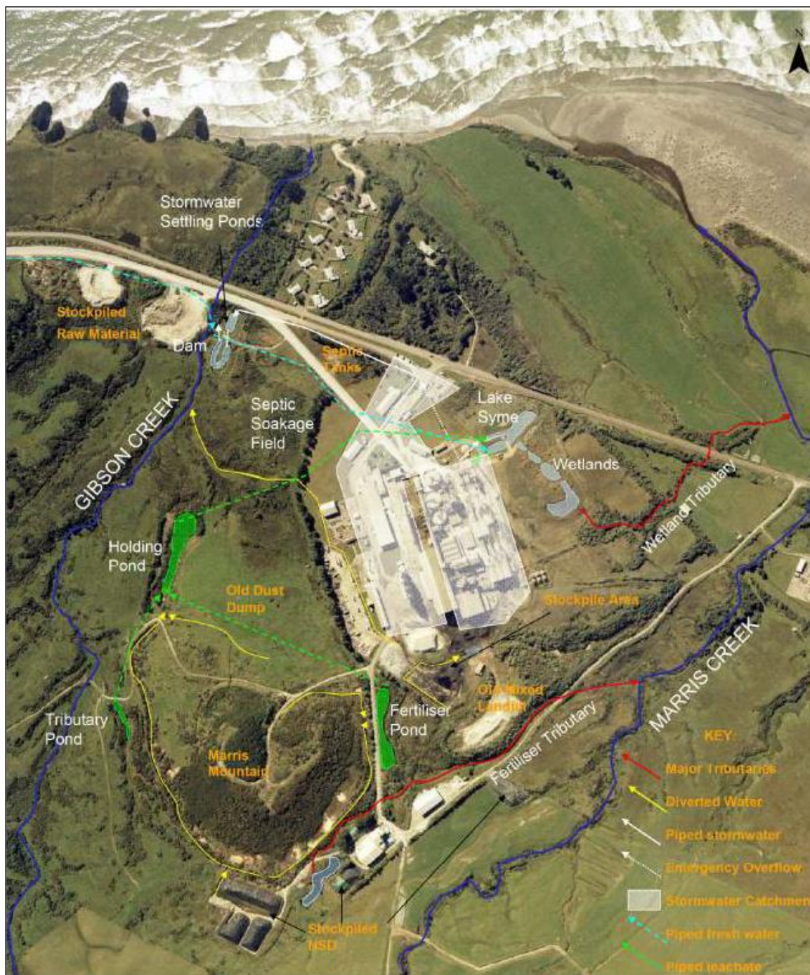
Figure 5: Water Management System
