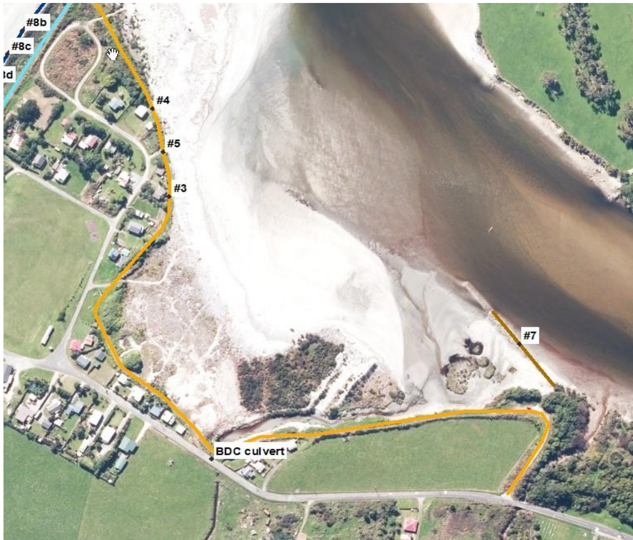
Map 6: Rating District stopbank (yellow line), culverts and rock work at Nos #3-#5, old groyne at No #7, and hardfill and dump site at bush area near landward end of old groyne - south bank of the Mohikinui River
