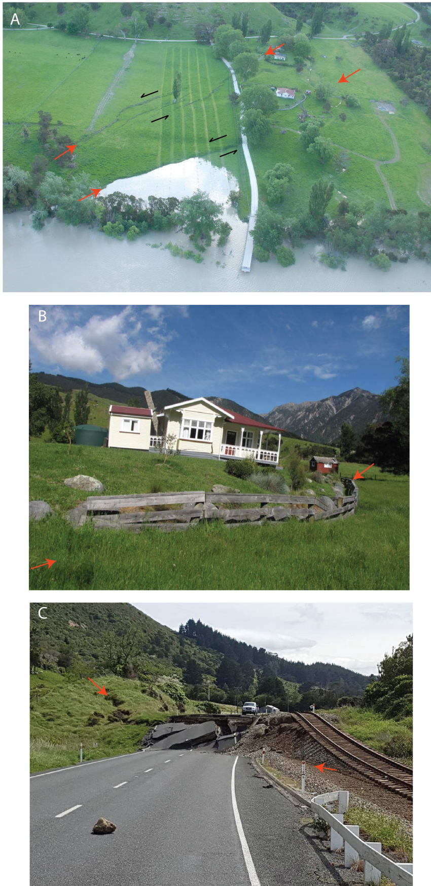
Figure 6.3 Photos of surface rupture along the Papatea Fault in the 2016 Kaikōura earthquake. (A) Distributed zone of surface rupture at Glen Alton; red arrows mark rupture traces. Black arrows show sinistral (left-lateral) sense of motion, also seen in bent tree rows. (B) Red-roofed house from (A), showing bending deformation on top of one of the rupture scarps. (C) Vertical deformation across SH 1 on the western strand of the Papatea Fault at the coast.
