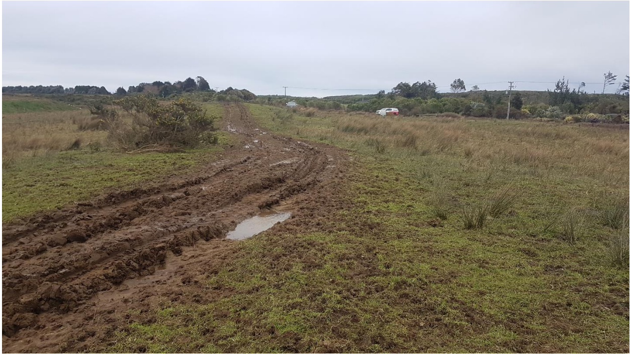
Figure 3. Photo showing typical ground conditions on site, these surface conditions are expected where shallow iron pan limits surface water from draining away
