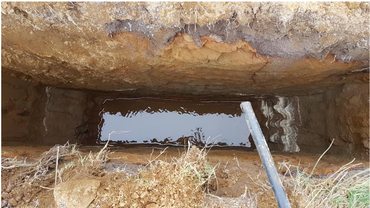
Figure 6. Photo of Falling Head Permeameter testing being undertaken
