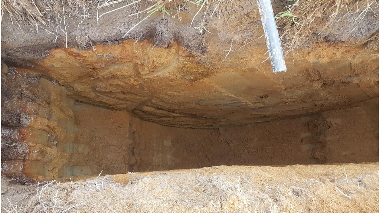
Figure 5. Photo of test pit at location P, underlying iron pan can be seen overlying sand
