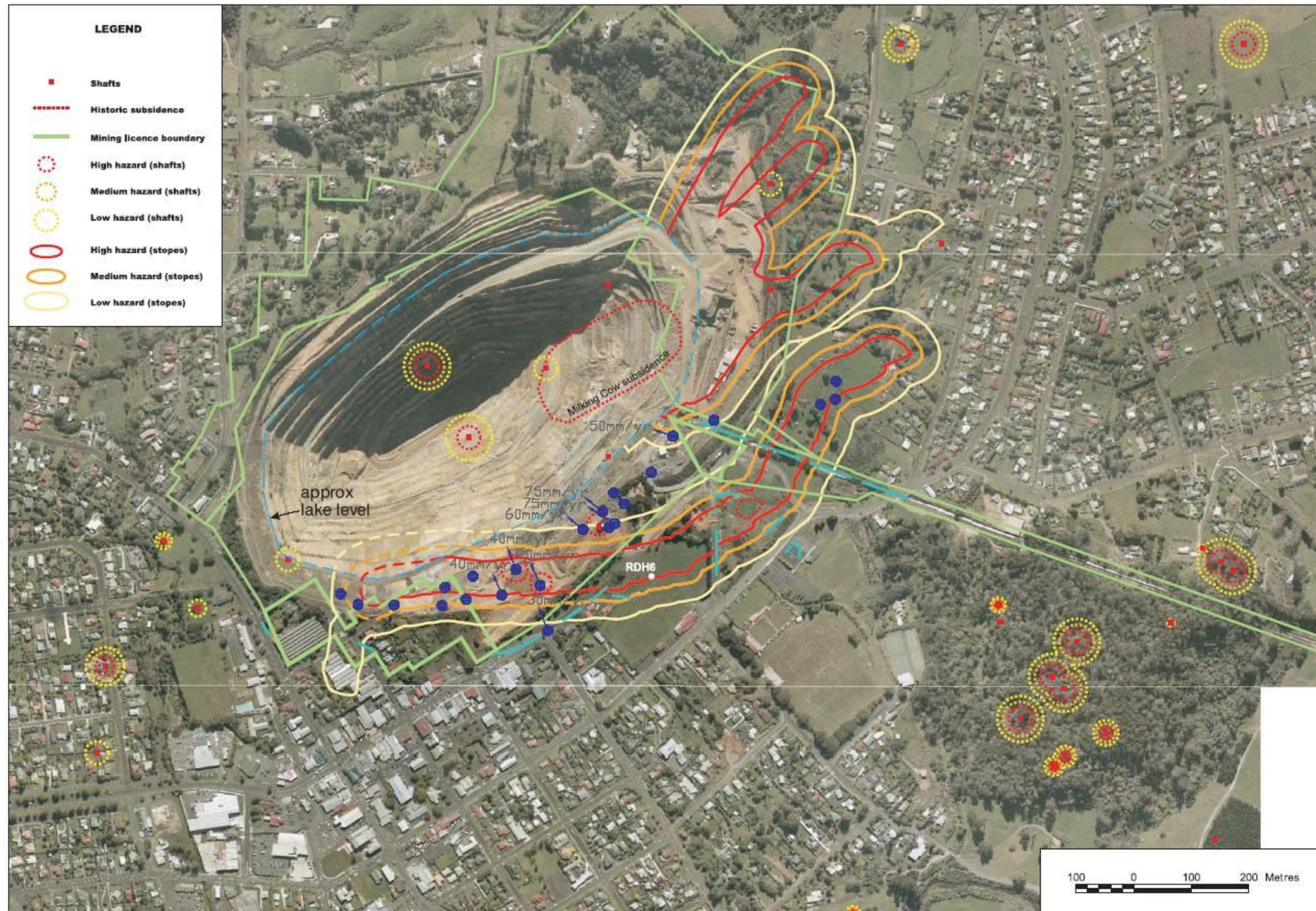
Figure 5: Aerial photo of Waihi showing collapse areas, the open pit and probabilistic hazard zones – circles around shafts, elongated areas above lodes (from the August 2002 GNS Report). The Edward South hazard zones were changed in the 2003 GNS report and 'Martha' stopes have been added - this report.
