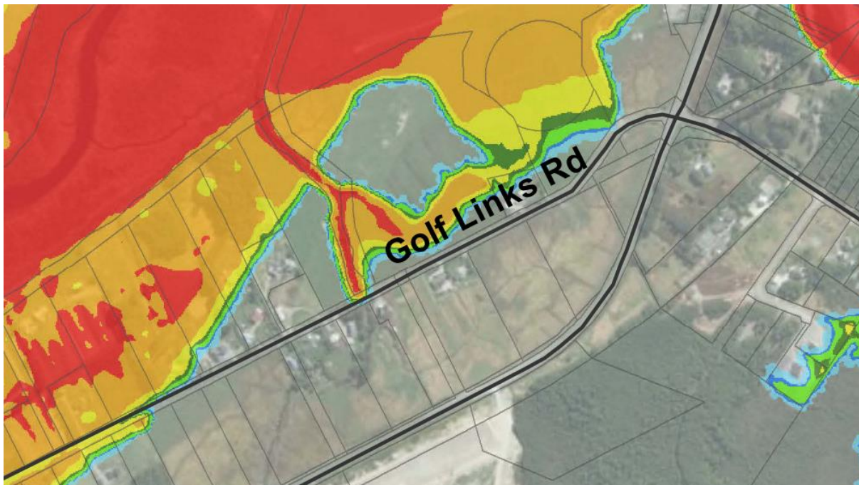
Figure 2. 1 in 100 year event including climate change (2100) RCP Scenario 8.5, 1.4m Sea Level Rise, 0.4m Storm Surge
