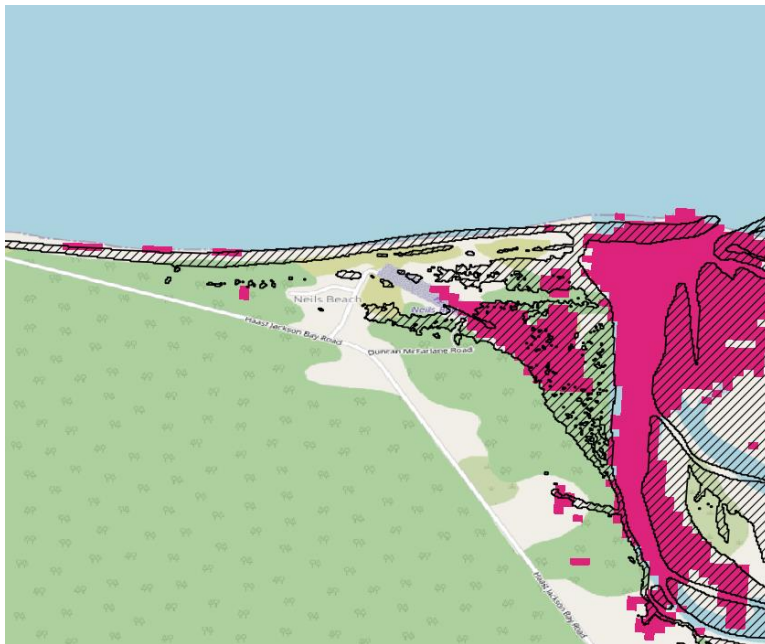
Figure 3-2: Inundation extent in Neils Beach based on SRTM and LiDAR DEM. The inundation extent based on SRTM (pink) does not see the smaller ponds or even the beach itself. The LiDAR-derived inundation extent (hashed) accurately sees ground level below the tree canopy and small inundation pathways.
