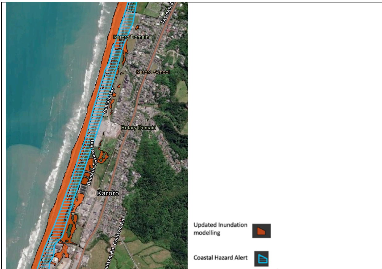
Figure 9: Comparison of TPP Coastal Hazard Overlays and Updated NIWA Inundation Modelling Karoro
