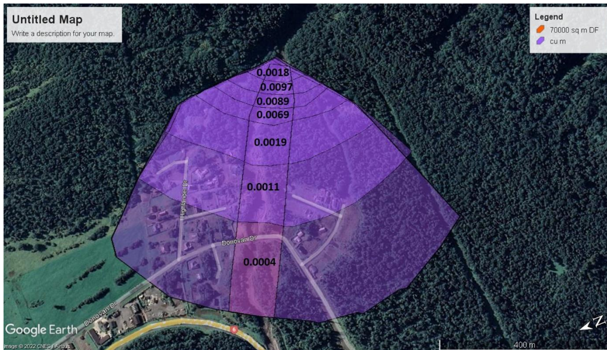
Fig. A2.5 Outlines of Stoney Creek debris-flow deposit areas with annual probabilities. Modified Google Earth image.
