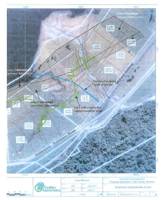
**Figure A.** Map showing suggested Fault Rupture and Deformation Avoidance Zones in the NE part of the Lake Poerua subdivision. The green line shows the expected seiche inundation level (from the lake) across this area. The blue line demarks the area covered by schistose fan debris.
