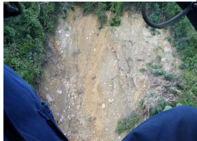
Figure 7. The headscarp of this landslide shows a gradual transition from disturbed to undisturbed ground and there does not appear to be a high likelihood of headscarp regression. Additionally, flattened vegetation within the landslide scar is likely to regrow quickly. Photo: BDC.
