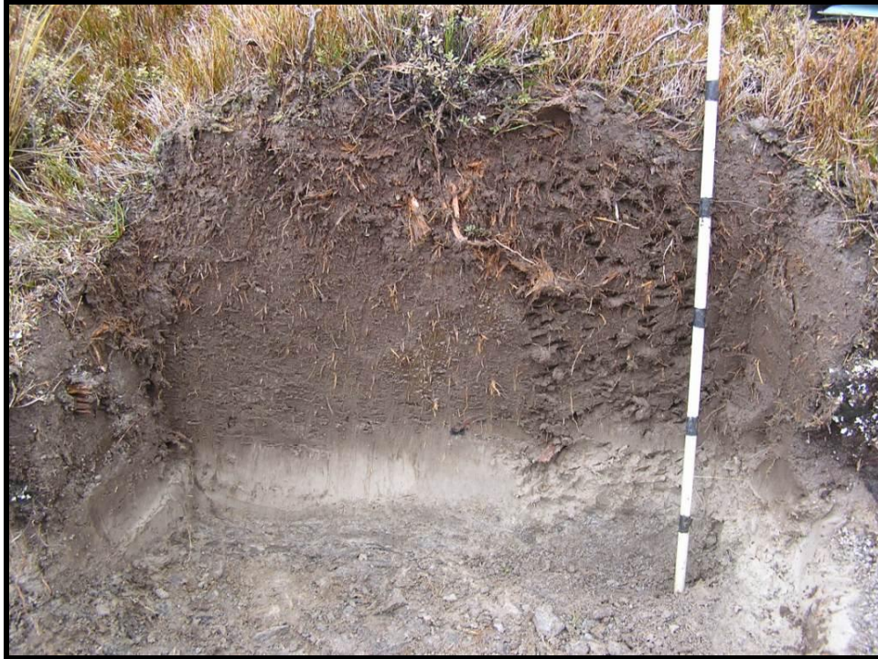
Figure 2. Trent soil profile (Ah1/Ah2/Br/R) with a gleyed subsoil over sandstone rock, a Gley Soil. Scale in 10 cm increments.
