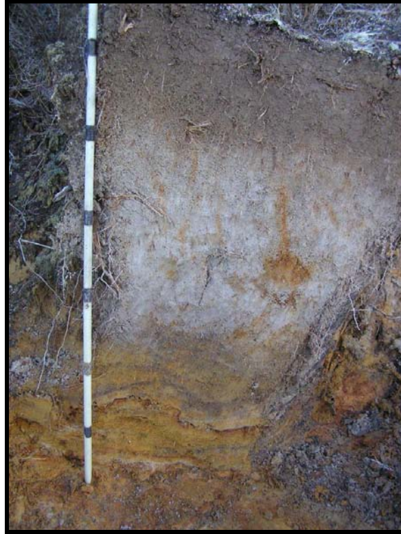
Figure 4. Denniston soil profile (Ah/E/Bhw/Bfm/Bs/R) of a Humus Iron Podzol. Scale in 10 cm increments.
