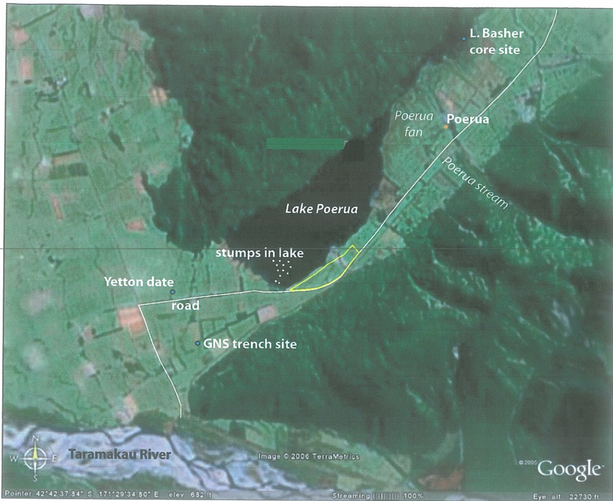
Figure 2 Satellite image view of the Inchbonnie-Lake Poerua area with key sites used for geomorphic interpretation of fault activity described in text. The area of the proposed subdivision shown in yellow. The Alpine Fault is not mapped on this image, but was trenched at the GNS site at Harris farm. Field boundaries W and NE of this site mark the approximate location of the fault.
