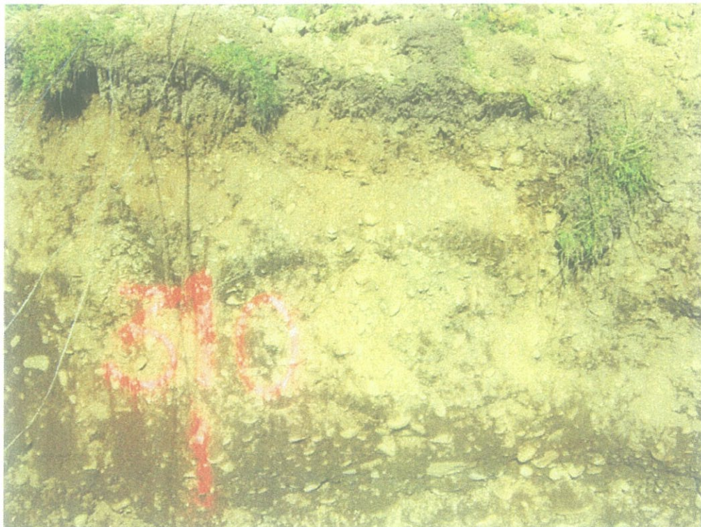
Figure A4: Compact brown slightly weathered sandy gravels at 30m in Trench A. Sediments locally bedded at this location, with suggestion of deposition as delta into body of water.
