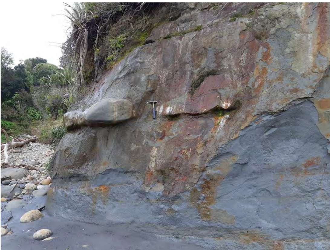
Site photo 7 Calcareous concretions (strength: moderately strong) observed in the mudstone on the beach by Gibsons Creek outlet.
