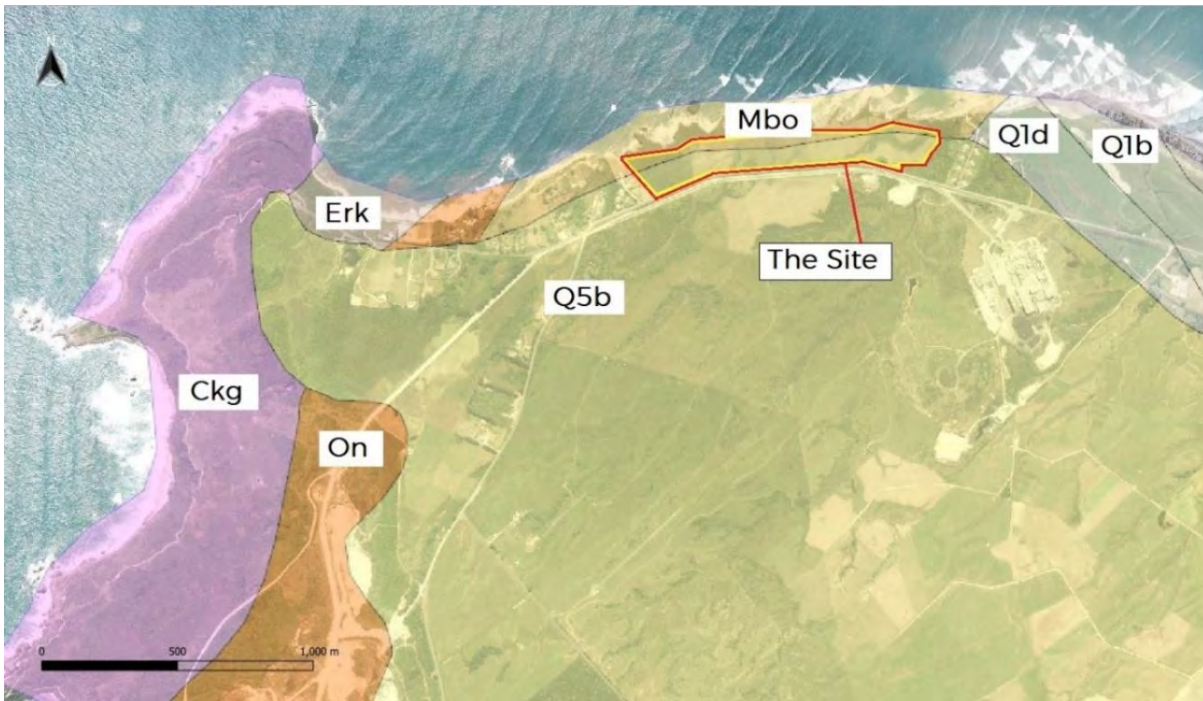
Figure 3 Geological map of the Cape Foulwind area, which indicates that the site (outlined in yellow) is dominated by Miocene age blue-grey, micaceous muddy sandstone of the O'keffe Formation (Mbo) overlain by a thin cover of Quaternary marine sands and gravels of the Waites Formation (Q5b).
