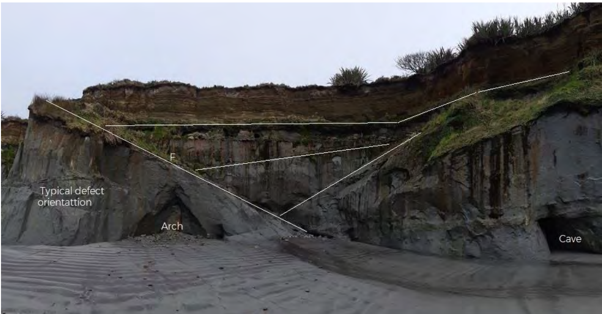
Site photo 5 Structural complexity observed in the mudstone from the beach. Likely low angle thrust fault (F) with a small drag on the hanging wall block (RHS of photo) truncated by erosional unconformity and overlain by Quaternary sands and gravels. Although the area appears relatively stable it shows potential for a range of failure modes including larger complex failures, block slides.
